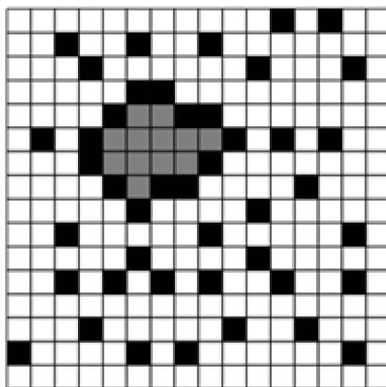
The empty zeolite pores (white) become clogged by coke (black). Once an area (grey) is surrounded by clogged pores, it becomes inaccessible and inactive, despite not being blocked
